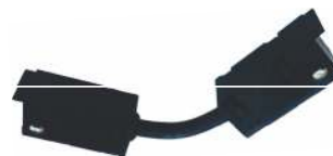
OP-826 SHORT CONNECTOR 2 PIN VOLTAGE : AC220V. DC48V HOUSING : MATT BLACK MATERIAL : COPPER+PC SIZE: 15 CM WIRE
